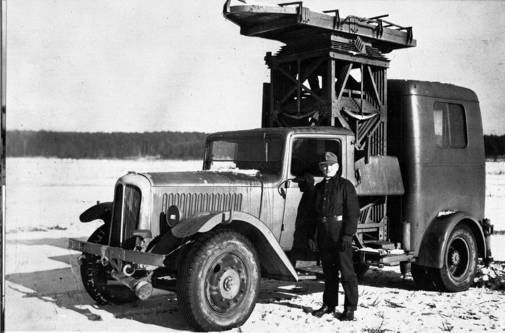
Tower truck of an FR battery with hydraulic platform for further servicing of the vertically erected rocket.(M)
